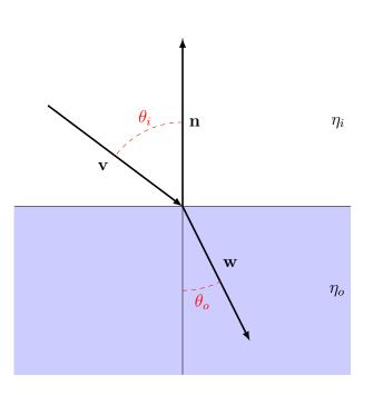
In the figure above, a ray originally in the air (index of refraction  $\eta_i$ ) enters a transparent material (index of refraction  $\eta_o$ ). The ray enters along direction  $\mathbf{v}$  and leaves along direction  $\mathbf{w}$ . You are given that  $\|\mathbf{v}\| = 1$  and  $\|\mathbf{n}\| = 1$ . You will construct  $\mathbf{w}$  such that  $\|\mathbf{w}\| = 1$ .  $\mathbf{w}$  lies in the same plane as  $\mathbf{n}$  and  $\mathbf{v}$ .
